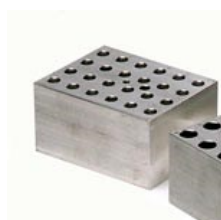
2524-0000 24-place block holds 0.5 ml tubes. Measures 3" W x 3.75" D x 2" H.
